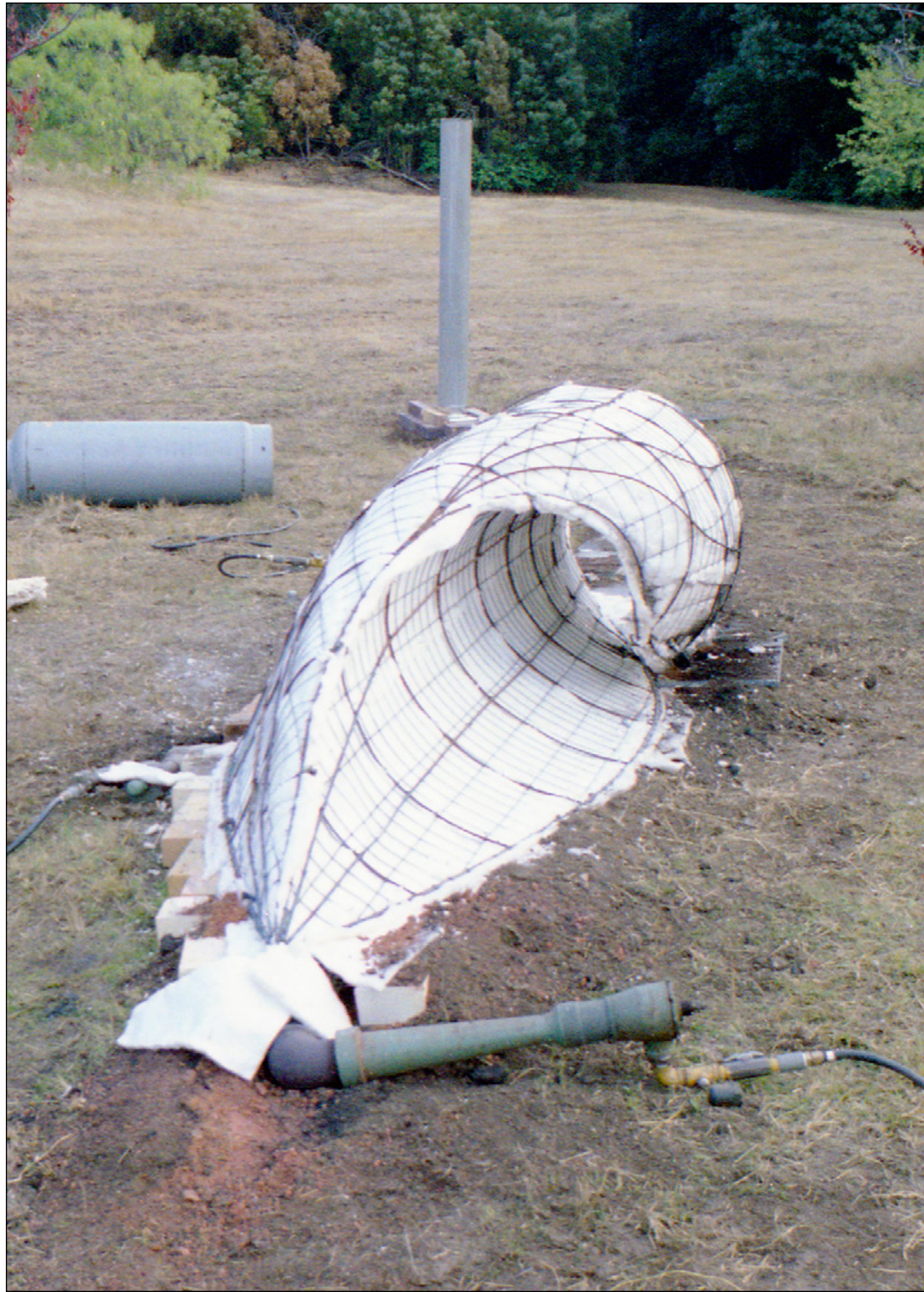
Fig. 74. Wave Kiln I (post fire state), 26 ft. long, ceramic fiber blanket, steel, propane, brick, Mills College, 1981.
