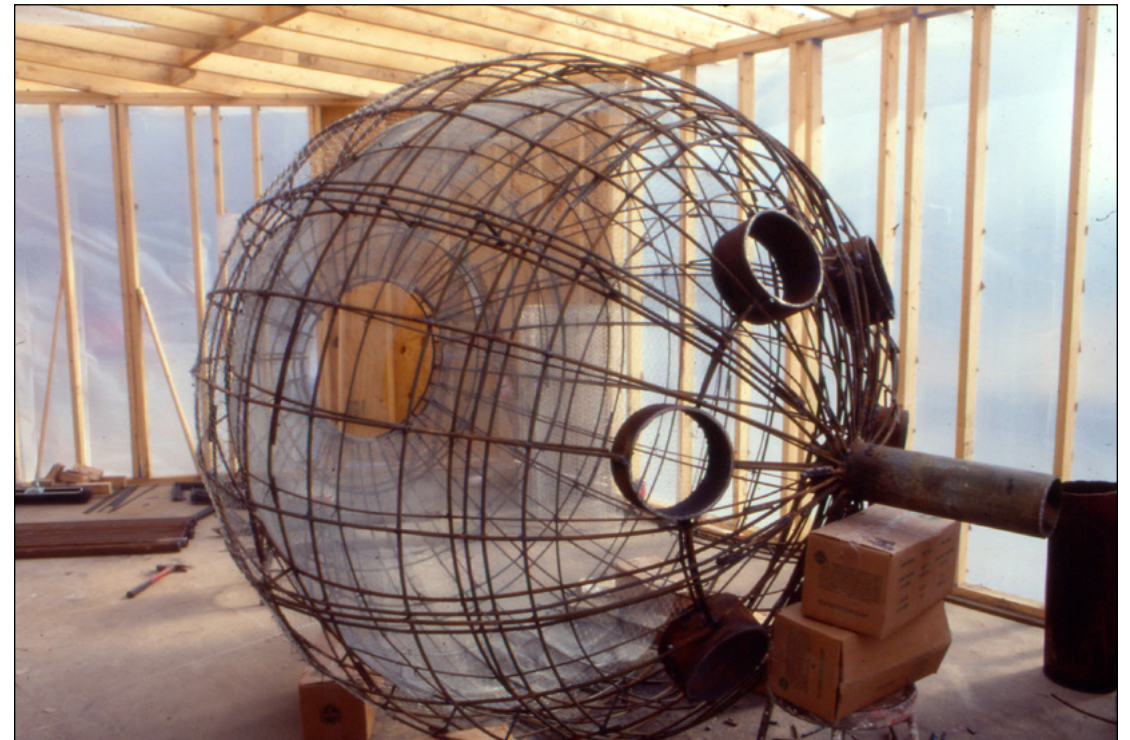
Fig. 194. Fabrication of Furnace , sphere, 6 ft.. dia., steel, galvanized mesh.
