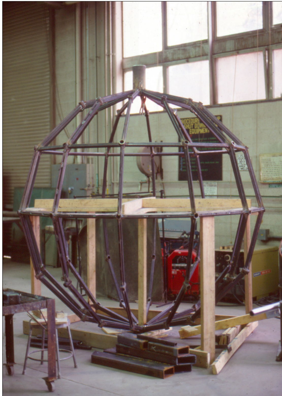
Fig. 193. Fabrication of Greenhouse , Tyler School of Art Sculpture shop, 8 ft.. dia., steel, wood.
